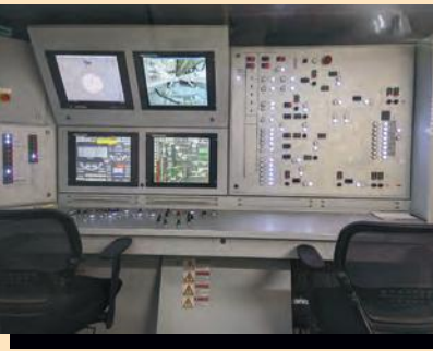
[ABOVE]: ■ The TBM operator monitors all operations from the control room. ■ Multi-service vehicles are used to transport the tunnel segments to the TBM. ■ The segment feeder brings in tunnel segments as the vacuum erector awaits overhead, preparing to move each segment into place. ■ The TBM has 54 hydraulic thrust cylinders that push against the tunnel ring to move the TBM forward.
