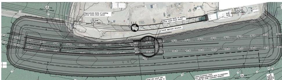
The North Trestle structure to support the roadway and Movement of Traffic (MOT) temporary deck and roadway will be constructed by installing piles. During the construction efforts (pile driving), water quality monitoring will be conducted.
