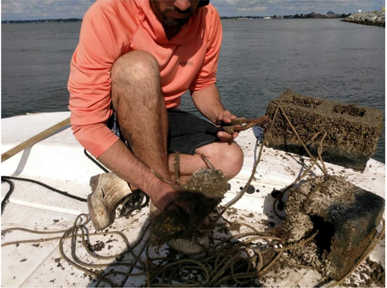
Figure 2. Picture showing biofoul and why the receivers needed to be downloaded so frequently. Most of the year there was little biofoul but during the summer (August 2017 pictured above) there was biofoul accumulation, which can decrease the tag detection range if not removed regularly.
