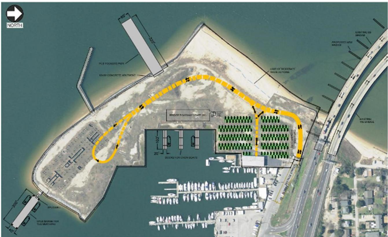
The existing bulkheads on the inside of Willoughby Spit will be repaired and three new piers will be constructed to provide access for crew boats and similar-sized vessels. (Appendix G – Attachment 1, Sheets 19 and 20).
