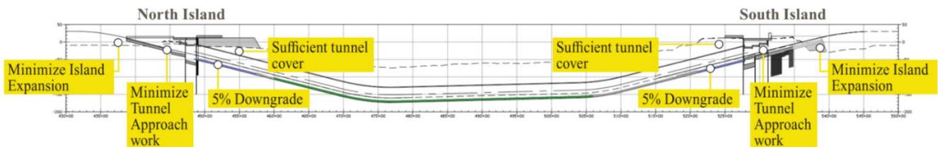
At these depths, the geology varies between loose to stiff cohesive material, traversing different combinations of mixed-face conditions. The TBM will also have to bore through areas where there are different types of ground improved areas. Bored material removed from the face of the tunnel will be amended with bentonite and pumped hydraulically to a Separation and Treatment Plant (S&TP) located
